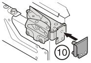
Fit the equaliser trim 9 in the recesses on the retainer.
