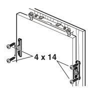
2. Slide the fitting aids ④ up level with the unit door: underside of stop edge of fitting aid = upper edge of unit door.
