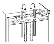
Screw the appliance door onto the unit door through the attachment brackets.
